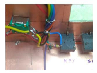
Leave the violet wire (The A7). Keep it coiled. It is not used in the  $\mu BITX$ . If you can hack your way around the  $\mu BITX$ , find some use for it.
