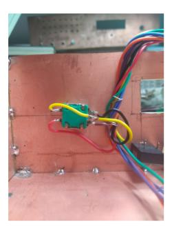
The encoder has three tabs on one side that correspond to Encoder's A, ground and B tabs. On the other side is the push switch. It has to be wired as follows:
