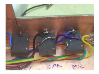
Tip: You can connect a speaker by connecting an internal speaker to the ground lug and any of the two unconnected lugs of the headphone socket.
